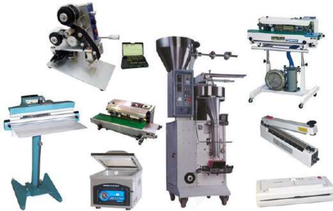
Contoh beberapa mesin pengemasan: Continuous Band Sealer , Hand Sealer , Vacuum Portable , Pedal Sealer , Coding Hot Print , Continuous Sealer with Gas Filling , Mesin Kemasan Renteng, dan lain-lain.
